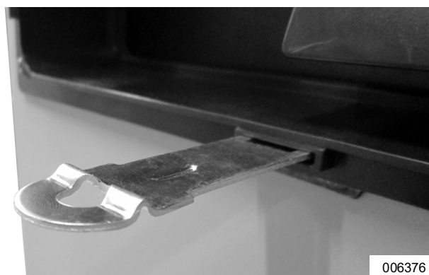
Figure 3-7. Install Viewing Window Hasp
